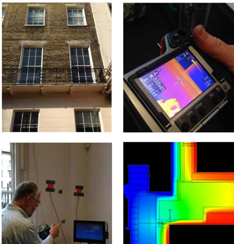
Thermal monitoring of the retained facade on the Park Crescent West project established that the thermal conductivity ( $\lambda$ -value) of the existing brick was below the default value, enabling the designers to achieve a slimmer wall build-up. Heat flux analysis (by Eight Associates) identified that isolators would be required on the restraint brackets to minimise thermal bridging.
